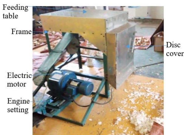
Fig. 12 - Electrical motor-driven cassava slicer
