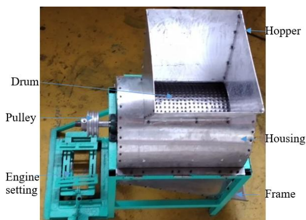
Fig. 5 - Corm pulverizing machine
