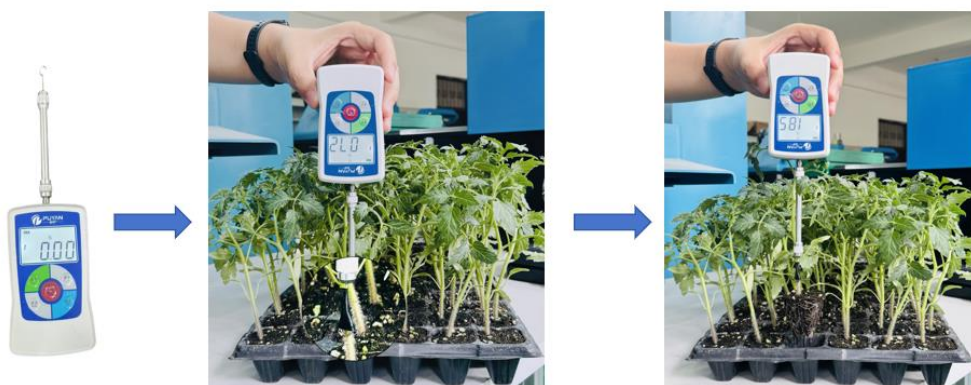
Fig. 5 - Extraction force measurement after and before vibration
