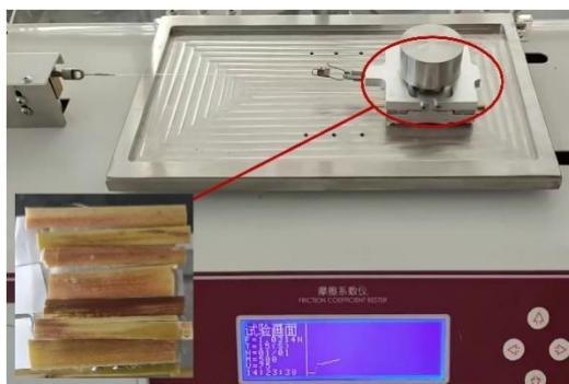
Fig. 4 - Friction coefficient measurement
