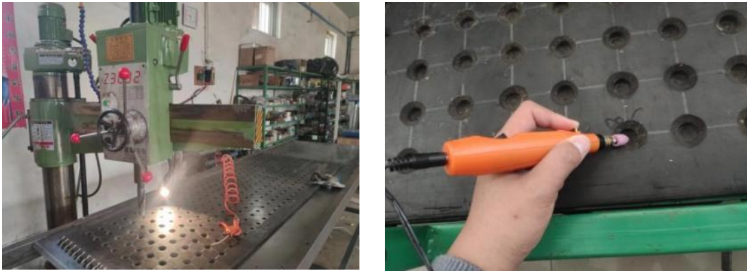
Fig. 3 - Drilling and chamfering of metering cells (a); forming of the hemispherical bottom (b)
