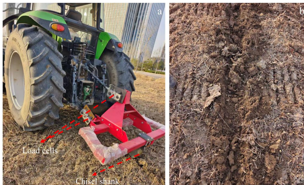
Fig. 7 - Measurement of draft force for the chisel shank operating in cohesive, salt-affected soil in the Yellow River Delta: (a) experimental setup and (b) the resulting furrow profile
