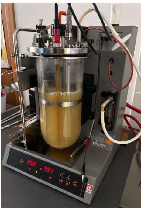
Fig. 1 – Macroscopic view of the Saccharomyces cerevisiae culture broth in the Minifors 2 bioreactor
