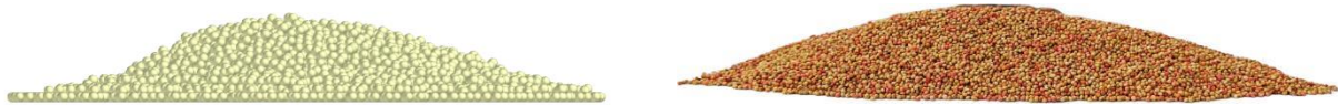
Fig. 8 - EDEM simulation of seed pile formation and photograph of the seed angle of repose.
