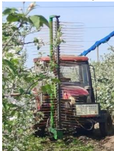
Fig. 3 - Field operation of the orchard flower-thinning machine
