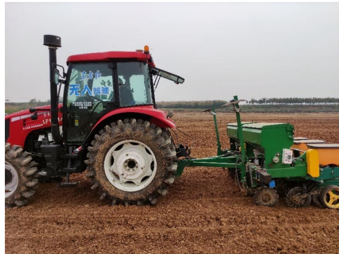
Fig. 11 - Field experiment of sowing operation control accuracy
