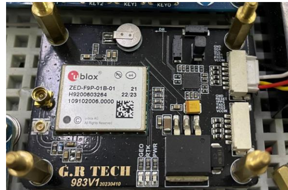
Fig. 3 - ZED-F9P High-precision positioning board
