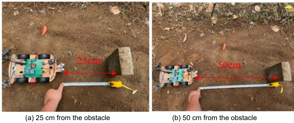
Fig. 8 - Ultrasonic ranging results in Scene 3
