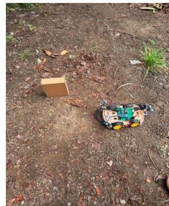
(f) Ultrasonic detection indicating that the distance from the obstacle was greater than 30 cm
