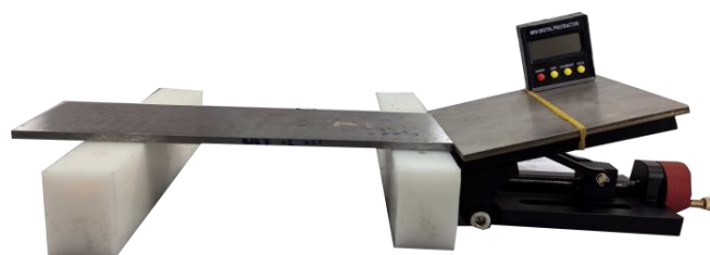
Fig. 5 - Experimental Equipment for Inclined Plane Rolling Method 2
