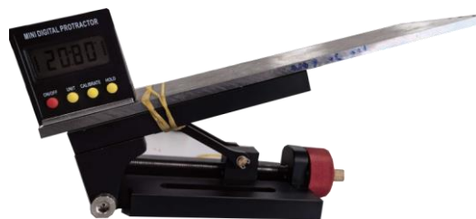
Fig. 4 - Experimental Equipment for Inclined Plane Rolling Method 1
