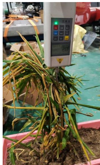
Fig. 6 - Process of ginger stalk pull-out force test
