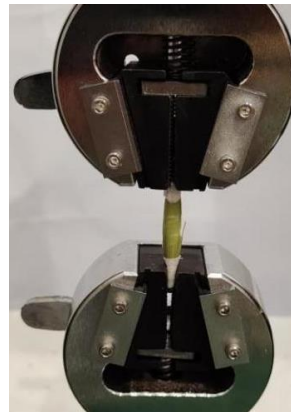
Fig. 5 - Process of ginger stalk tensile test
