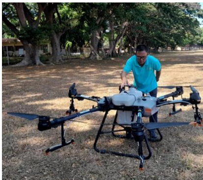
Fig. 1 - Machine inspection of RPAS Agricultural Drone (DJI Agras T30)
