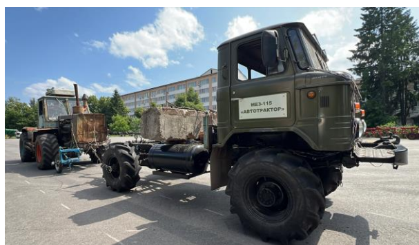
Fig. 2 – Traction tests of the “Avtotractor” on an asphalt concrete surface
