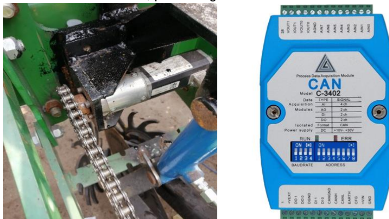
Fig. 4 - Split-type electric drive solution a) Brushless DC motor type BG45×15SI; b) CAN analogue output module
