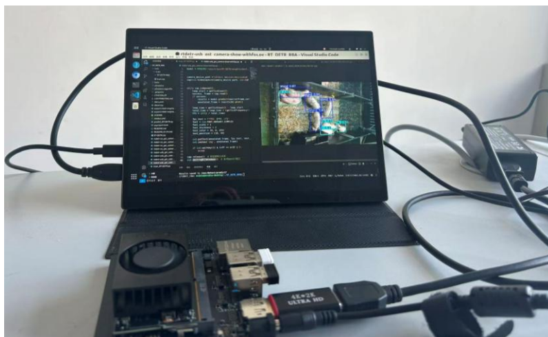
Fig. 13 – Deployment and inference verification of RAFE-DETR on the NVIDIA Jetson Orin NX Super platform
