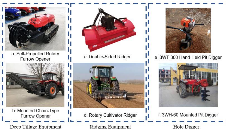
Fig. 5 - Pre-planting site preparation equipment
