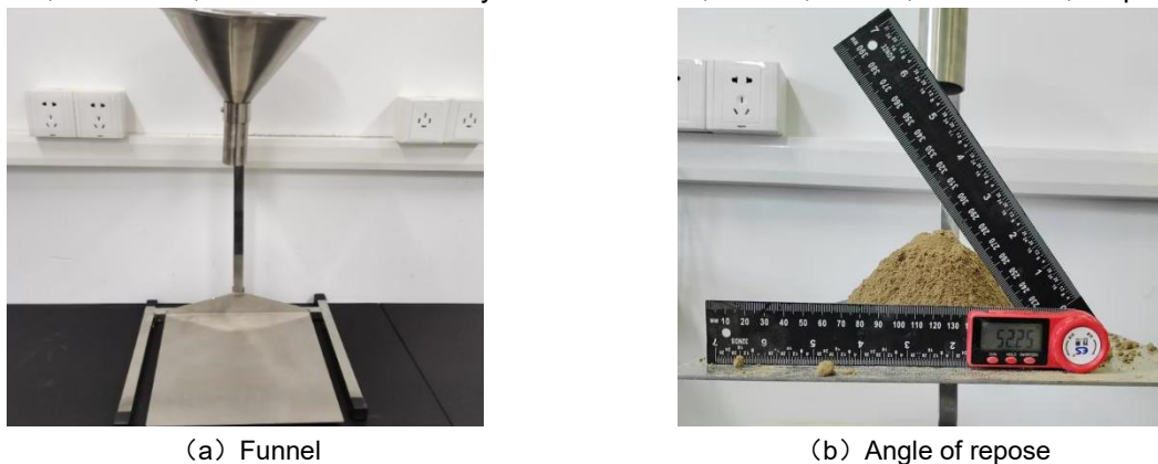
Fig. 2 - Stacking angle measurement test
