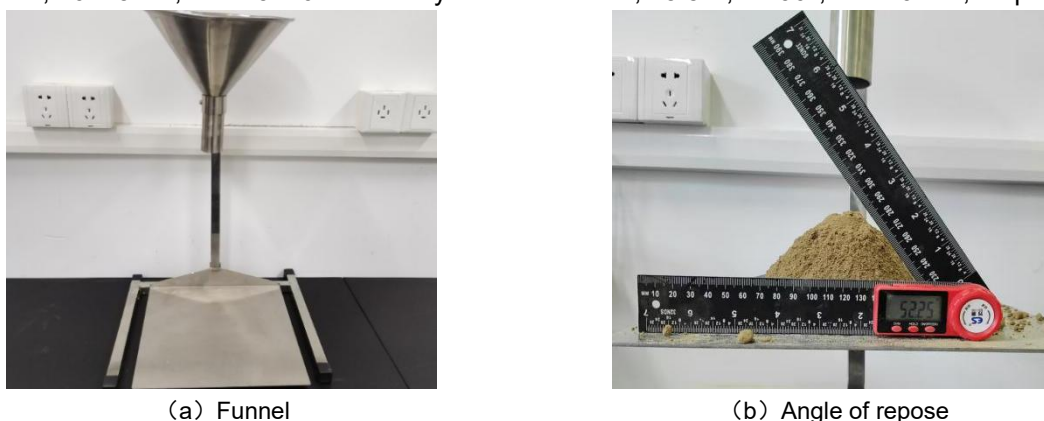
Fig. 2 - Stacking angle measurement test
