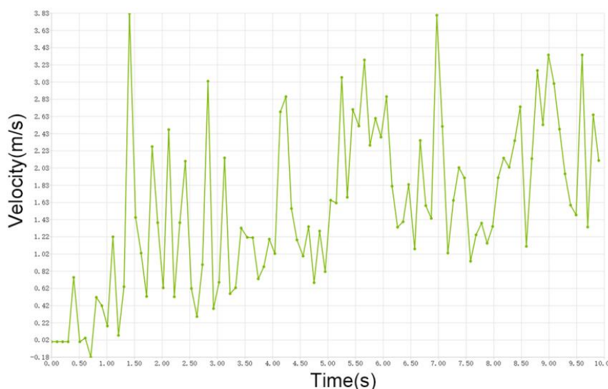
Fig. 3 - Axial velocity distribution map from the EDEM simulation
