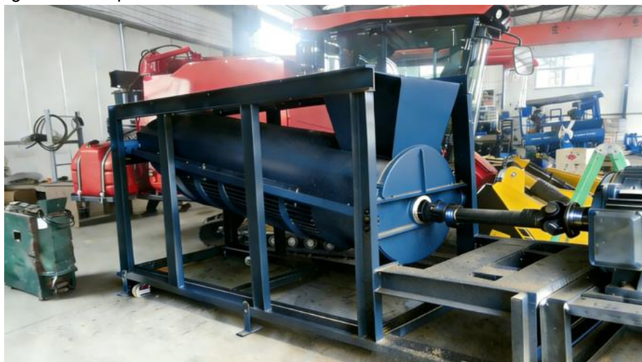
Fig. 7 - Modular axial-flow corn threshing and separation device test bench
