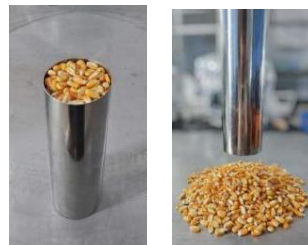
Fig. 6 - Physical test procedure for the formation of a corn kernel pile
