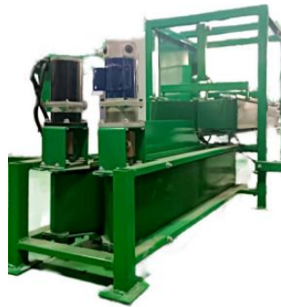
Fig. 12 – Experimental test rig of belt-type potato stubble clamping and pulling device
