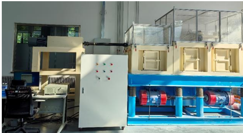
Fig. 2 - Wear performance testing machine for agricultural machinery tools
