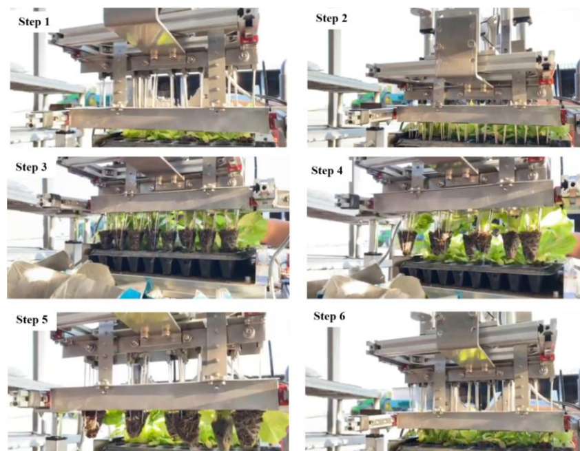
Fig. 9 - Main operating steps of the seedling feeding control program
