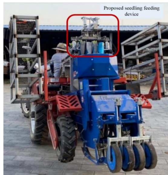
Fig. 1 - Single-disc vegetable transplanter equipped with the developed automatic seedling feeding device
