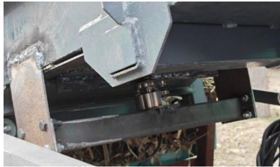
Fig. 3 - Pressure sensor installation diagram
