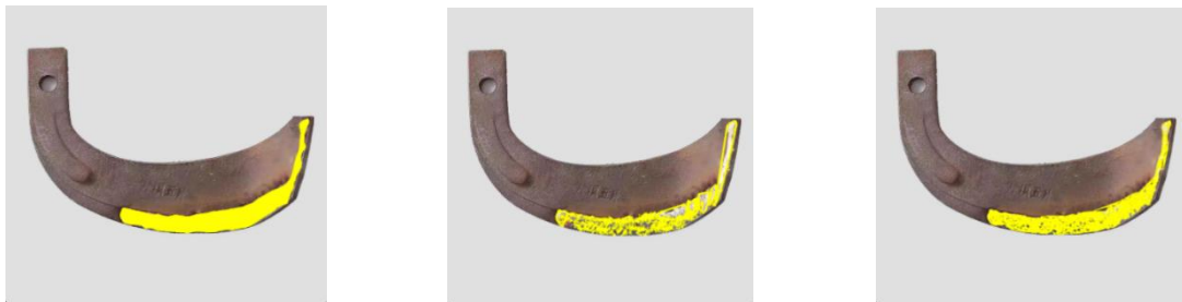
Fig. 7 – (a) Improved Alpha Shapes; (b) Convex Hull; (c) Delaunay partitioning and merging
