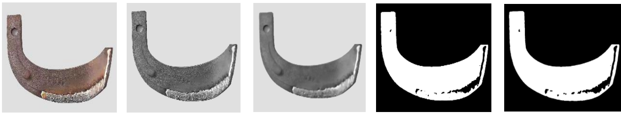
Fig. 1 – (a) Blade original image; (b) Conversion of greyscale images; (c) Gaussian blur; (d) OTSU Automatic Threshold Segmentation; (e) Morphological closure operation
