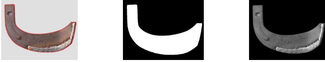
Fig. 2 – (a) Maximum area contour; (b) Mask processing; (c) Extract grayscale information from the object region
