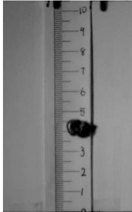
Fig. 6 - High speed camera calibration system of restitution coefficient
