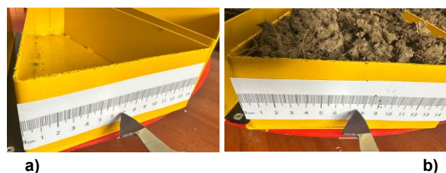
Fig. 8 - Images from container positioning error measurements (n=100 complete rotations)
