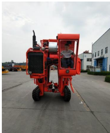
Fig. 7 - Straight driving test of tobacco harvester
