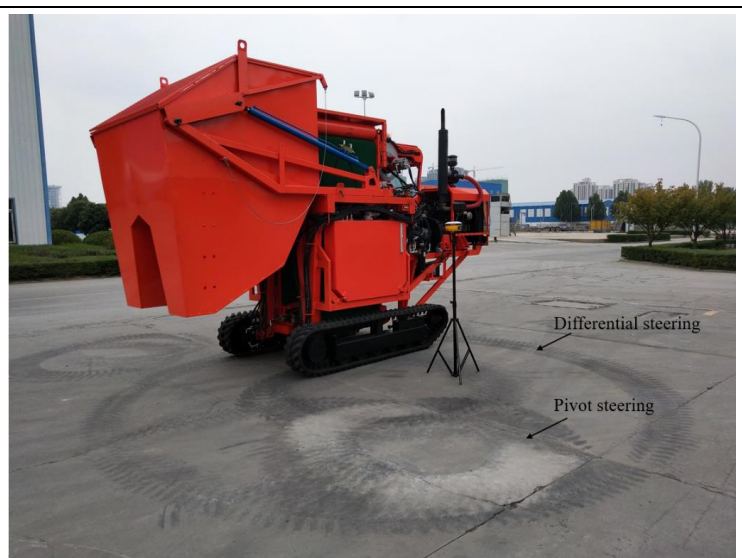
Fig. 10 - Steering test site of Tobacco harvester
