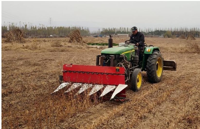
Fig. 9 - Field experiment on profile control of buckwheat windrower header
