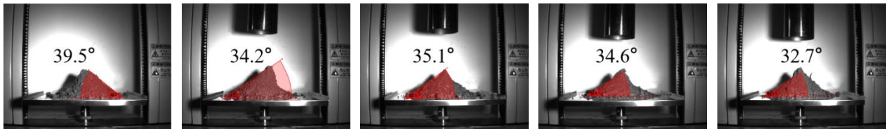
Fig. 3 Soil repose angle measurement
