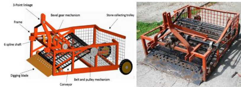
Fig. 8 a) Design schematic of the stone collector; b) Assembled stone collector (Rudani, M.R. et. al. 2018)
