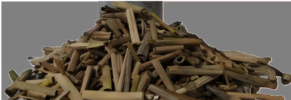
(b) Extraction of rice straw response angle boundary
