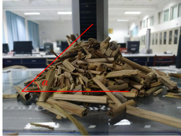
(a) Rice straw response angle test
