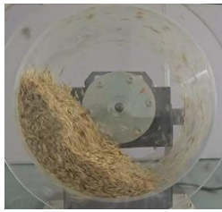
Fig. 9 - Physical experiment of dynamic angle of repose
