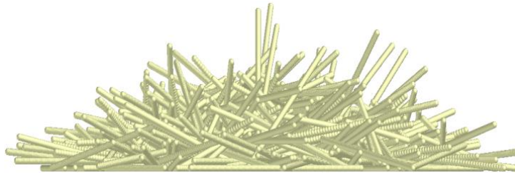
Fig. 3 - Simulation experiment of angle of repose for barley seedling stems
