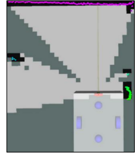
Fig. 27 – RViz screenshot of real-time visualization and distance measuring
