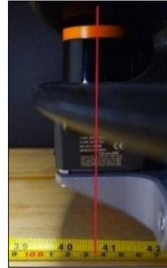
Fig. 26 – LiDAR accuracy validation
