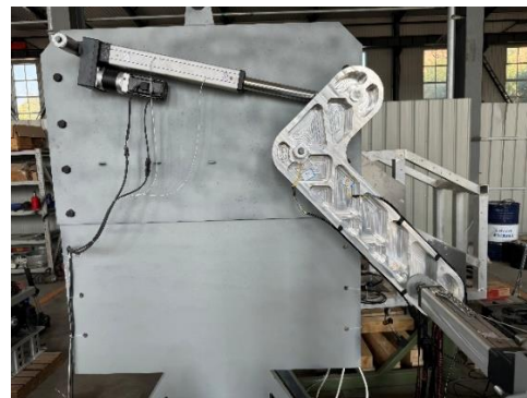
Fig. 15. Static test of front/rear arm specimen
