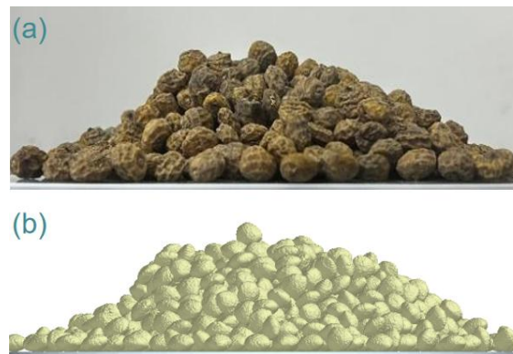
Fig. 14 - Simulation of stacking angle after parameter optimization of tiger nuts
