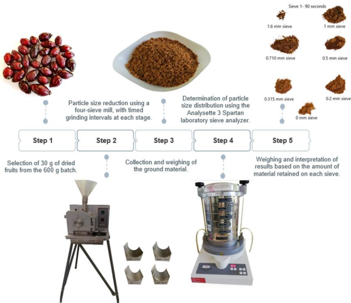
Fig. 2 - Experimental protocol for particle size characterization as a function of grinding time and milling sieve mesh dimensions
