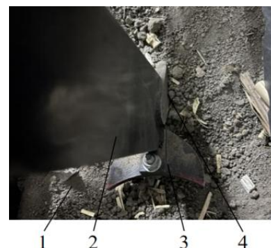
(b) Actual working conditions of subsoiler shovel in the tillage layer 1. Soil; 2. Shovel handle; 3. Shovel wings; 4. Shovel tip
