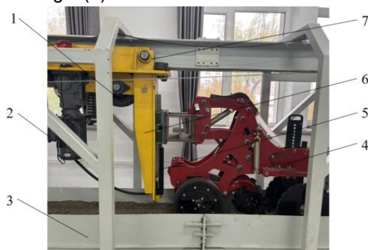
(a) Structural diagram of the pedestal 1. Travelling wheel; 2 Drive motor; 3. Soil tank; 4. Strip minimum tillage subsoiling fertilizer applicator; 5. Single-axis lifting mechanism; 6. Connecting arm; 7. Guide rail
