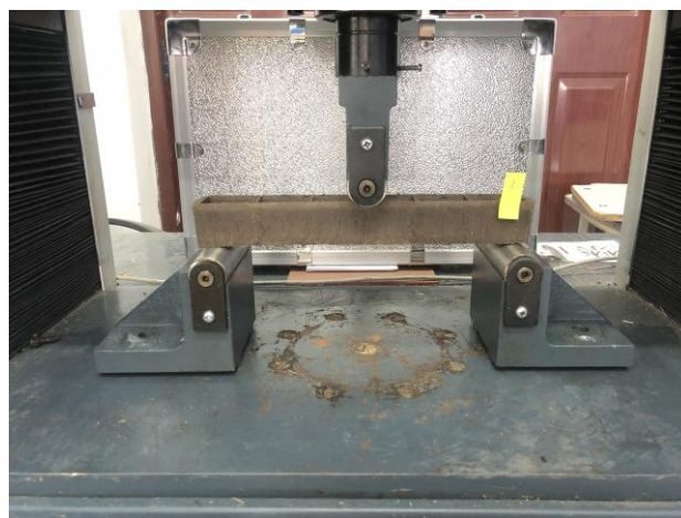
Fig. 3 - The flexural strength test of seedling trays using electronic universal testing machine
