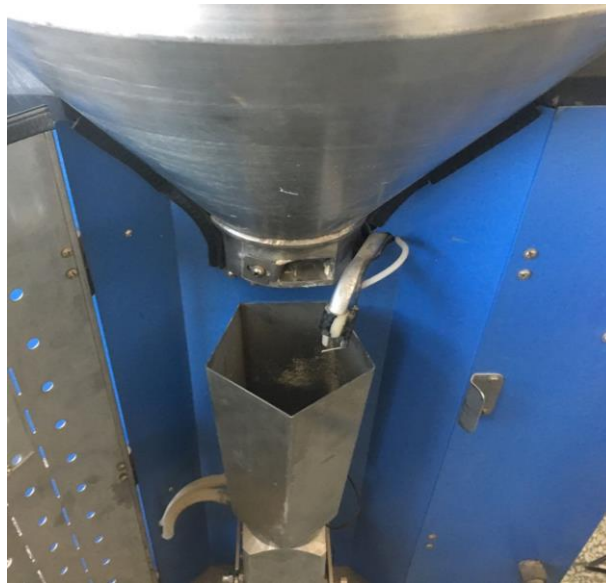
Fig. 8 – Milk replacer agitation mechanism with load cell
