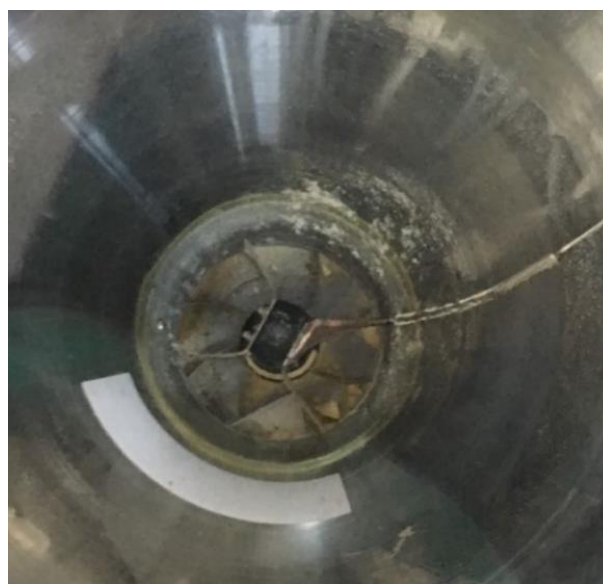
Fig. 7 – Circular-arc-8-blade conveying device with 45^\circ flow-guiding baffles
