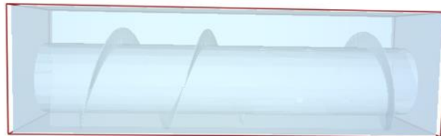
Fig. 4 - Simulation model of screw conveyor
