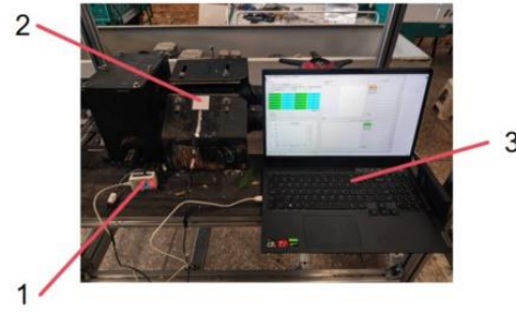
Fig. 6 – Schematic diagram of pressure test bench 1. Data display 2.FSR pressure sensor 3. Computer
