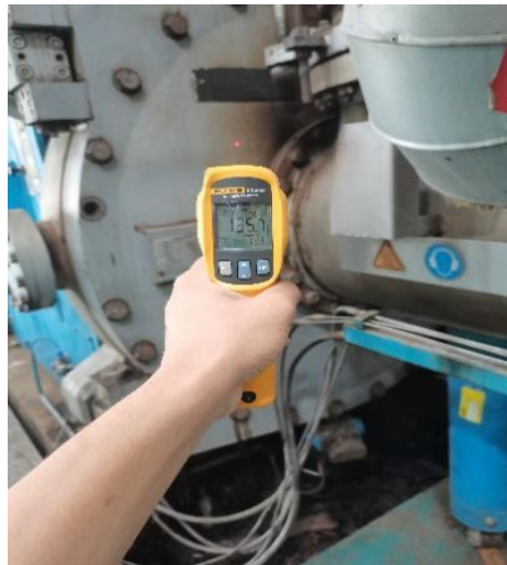
Fig. 3 - Temperature measurement of outer shell of grinding chamber
