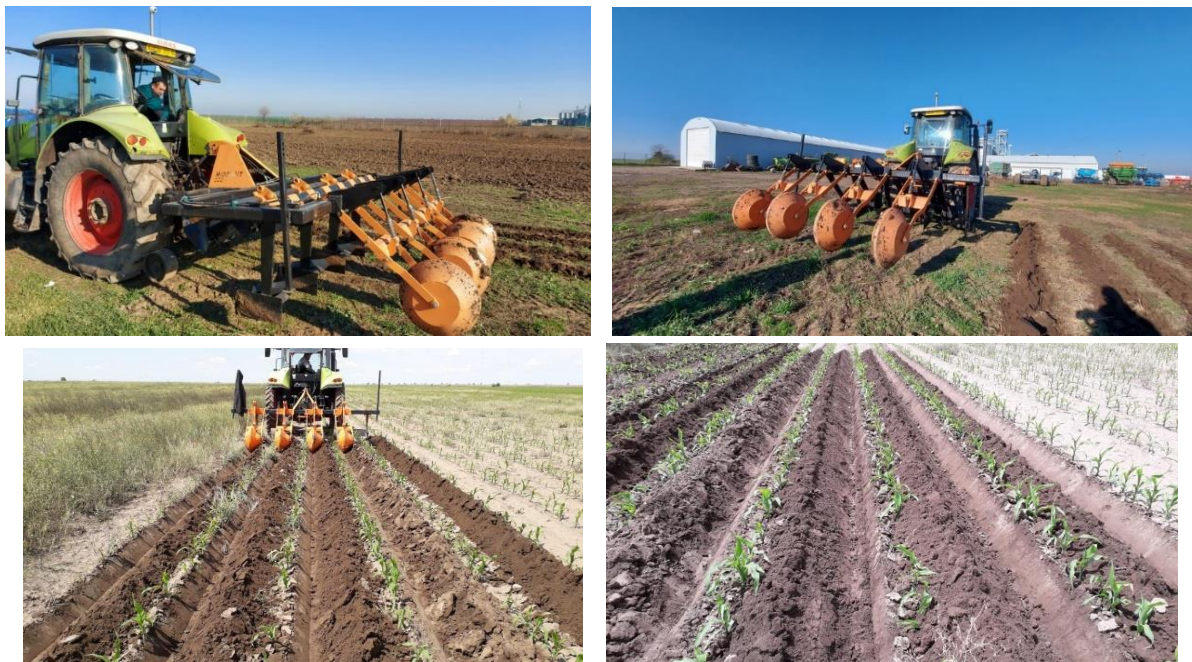
Fig. 2 - Aspects of an agricultural equipment for digging and tamping ditches for flood irrigation ( https://www.centruhidrauliccalarasi.ro/wp-content/uploads/2022/04/brazdar.jpg )
