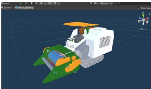
Fig. 7 - Virtual model of pepper harvester
