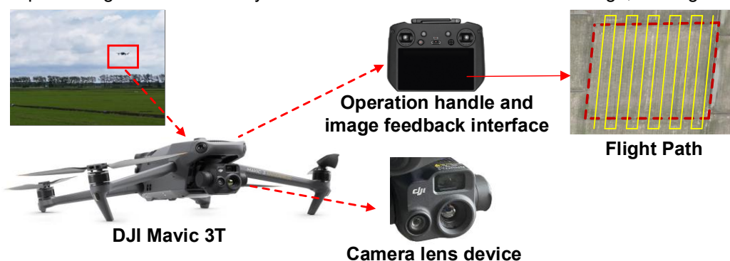
Fig. 1- Image acquisition equipment and range
